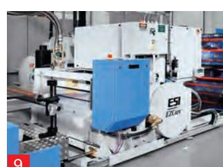
**9 Electron-beam curing**
