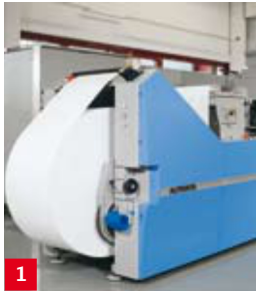
Unwind and infeed unit For rolls of up to 1270 mm/50" diameter. A servo drive provides the correct web tension.
