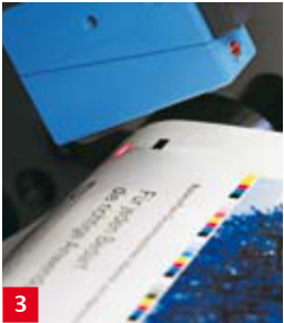
Re-insertion Integrated in the infeed unit for accurate, re-inserting of the web with sensors for the front and rear sides.
