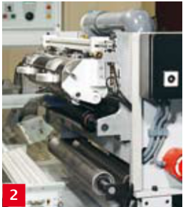
Corona treatment Plastic materials are pretreated with Corona to improve the adhesion of inks to the substrate.
