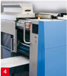
Ergonomic paneling Integrated paneling concept for optimum accessibility to the inking rollers without the need to dismantle covers.
