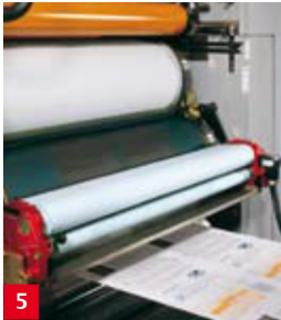
Blanket wash-up system The printing units are prepared for the attachment of a blanket wash-up system as standard.
