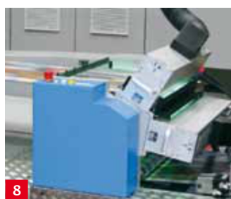
8 Cooling Station When temperature sensitive substrates are used, the UV heaters are mounted on a chill roller.
