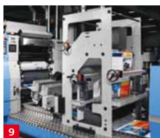
9 Register and Ink Control Automatic register control and in-line ink density control functions enable rapid setup times and optimum circulation stability.
