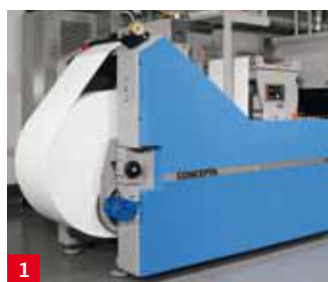
1 Unwind with Web Edge Control For rolls with a diameter of up to 1270 mm (50"). Re-insertion capability available.
