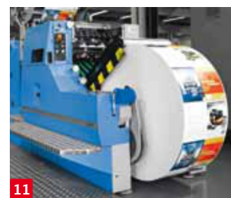
11 Rewind The electronically controlled web tension enables the processing of a broad range of substrates.
