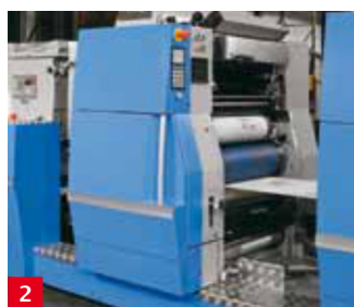
2 Printing Units Three application rollers and temperature-controlled oscillating rollers ensure optimum printing quality.
