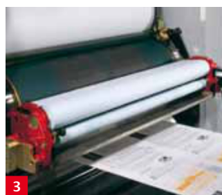
3 Blanket Wash-Up System As a standard feature, all printing units are designed to allow a blanket wash-up unit to be added.
