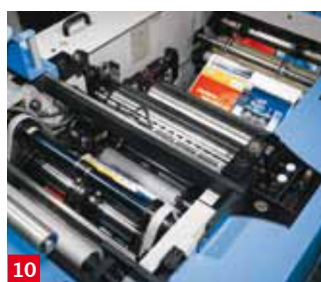
10 Processing Unit The convenient quick-set system and automatic register positioning for printing units result in short make-ready times.
